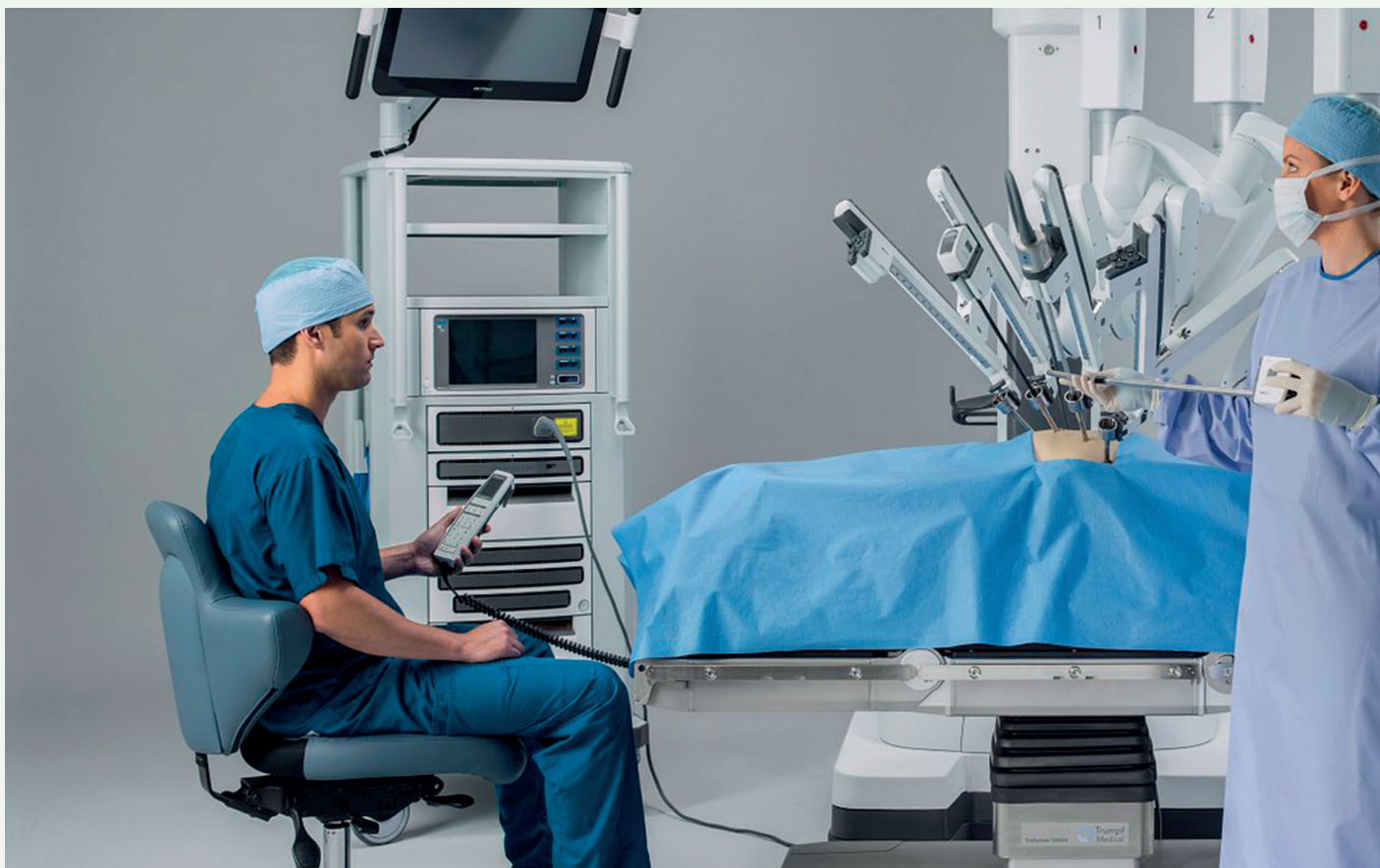
Robotic surgery for prostate cancer is performed with the surgeon in control at a separate console
